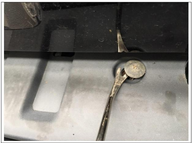
3. Remove 2x clips in front of grille with trim tool or flat blade screwdriver.
