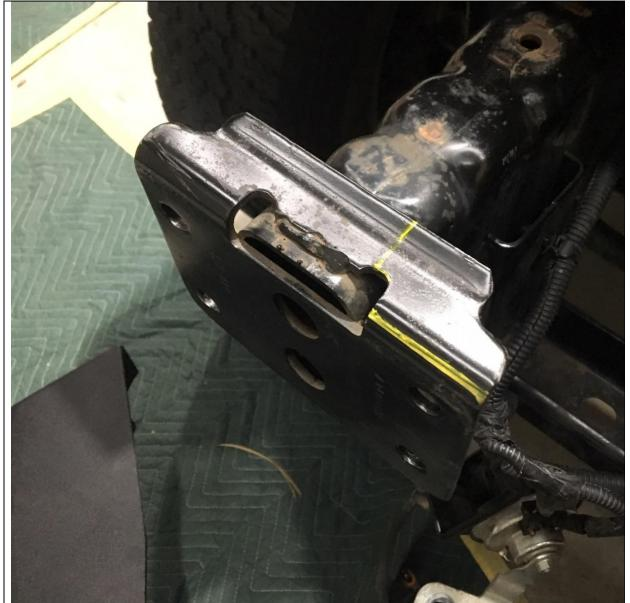
9. Depending on winch fitting you may need to trim part of chassis shown. Best is to test fit bull bar then drop winch in place and see if it contacts chassis.
