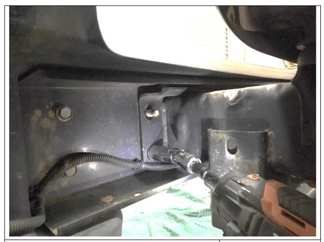
6. Remove 8x M10 hex nuts holding bumper on to chassis.
