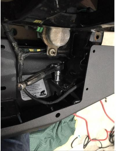
13. Put bull bar on to vehicle and use 4x M10x30 bolts, spring washers and flat washers to secure LHS to vehicle.
