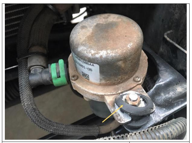
12. Also, winches will require the thread on the vacuum pump bolt to be trimmed. Drop winch on and see if it contacts this thread (most winches will not touch) If it does though, trim with angle grinder.
