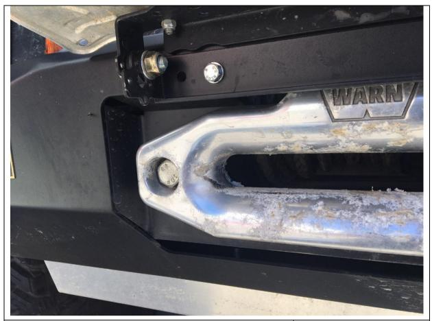
22. Fit winch fairlead as shown with hardware supplied with winch.
