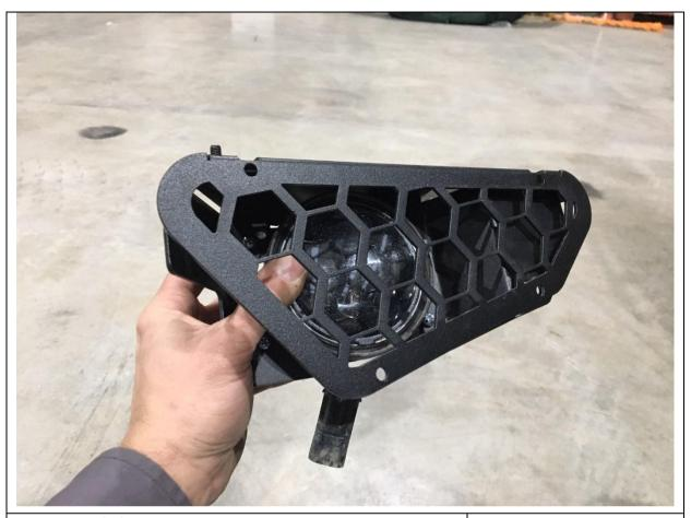
16. Next fit fog light bracket to mesh panel and secure with 1x M8x25 hex bolt, flat washer and flange nut on the top. The front will be secured through bar in next step.
