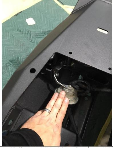
14. Re fit horn to original location on RHS chassis horn and use M10 bolts as per LHS. If fitting a winch push the horn down as far as possible with your hand bending its bracket.
