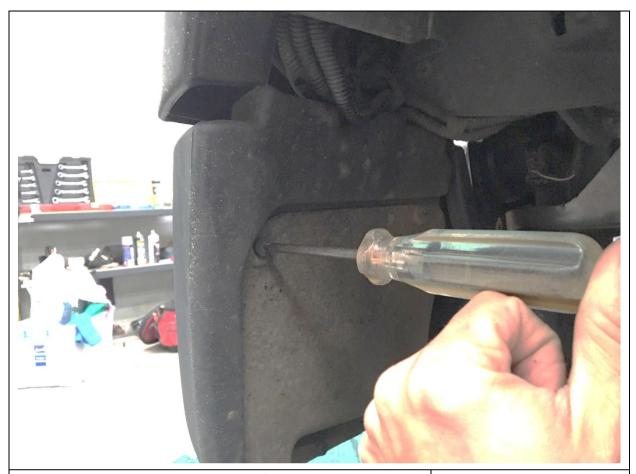
1. Start by removing screws behind fog lights
