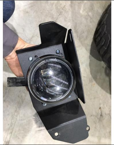
15. If fitting factory fog lights, do so now to supplied brackets using M4x12 pan head screws and flange nuts.
