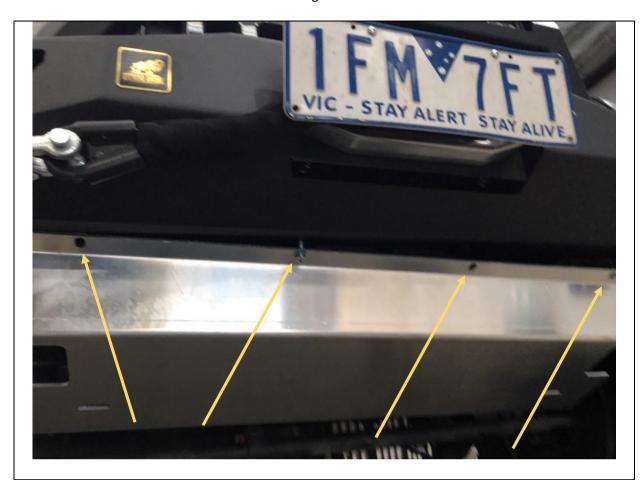
26. If fitting optional skid plate, hold plate up to bottom of bull bar and start the 4x M8x30 button head cap screws with washers to hold plate in place.
